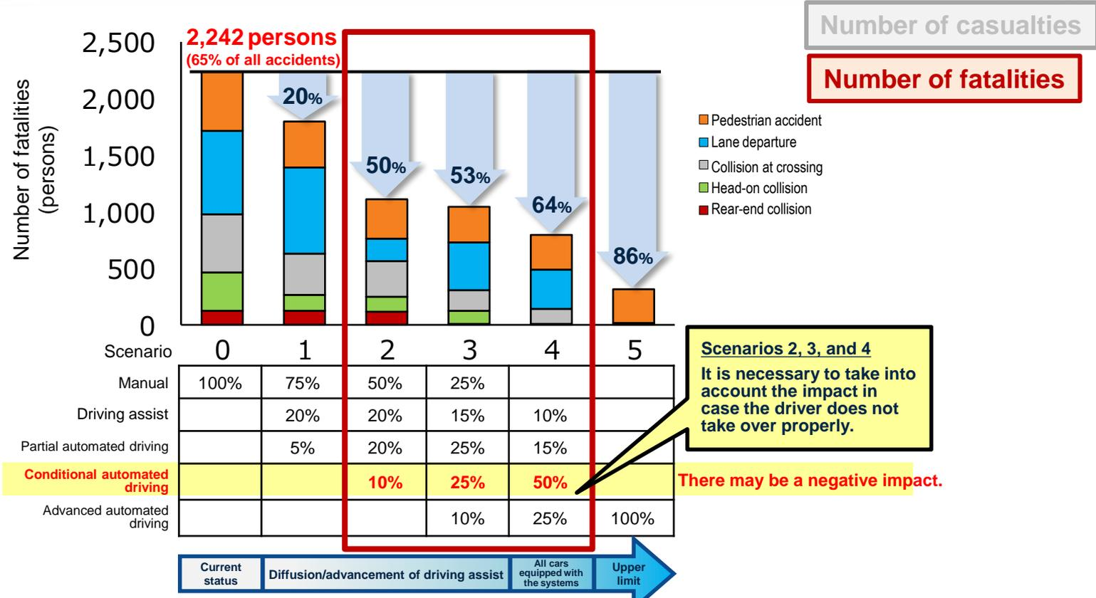
It was confirmed that the reduction effects at the national level can be calculated validly on condition that various automated driving systems diffuse in stages
