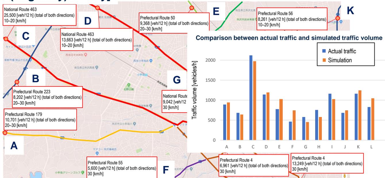
We confirmed that the traffic flow, which reflected the characteristics of traffic volume of 12 hours during the daytime at the main points within the scope of the simulation, was reproduced.
