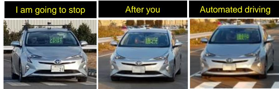
Experiment to simulate an external HMI on a test course
