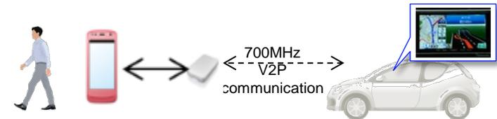
Proto type of pedestrian terminals and in-vehicle equipment with a view toward field operational tests
