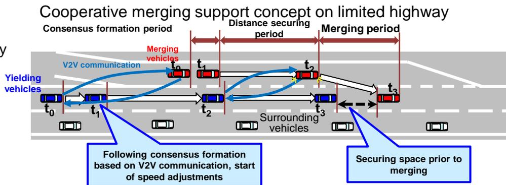
b. Examination of utilization of V2V and V2I communication in merging user case
