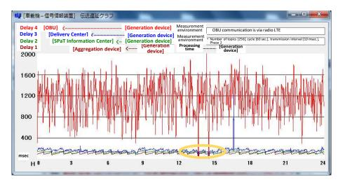
Continuous operation without MQTT-PING
