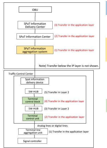
Verification point (1) The cause of the communication delay is assumed to be the transfer in the application layer.
