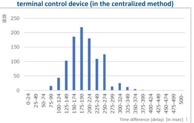
Communication delays between traffic signal controller and
