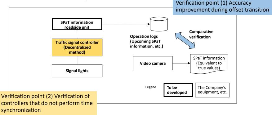
Supplementary information: Other than "adding SPaT information roadside unit" to the signal controllers currently in operation, the controller-based method can also be implemented by upgrading current signal controllers to those that support the method.
