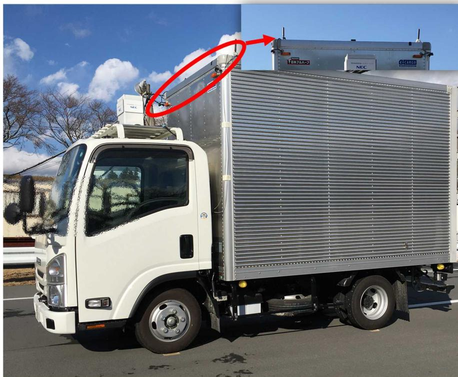
Fig. 3.4.1-2 Small truck equipped with OBU (radio antenna indicated by the red circle)
