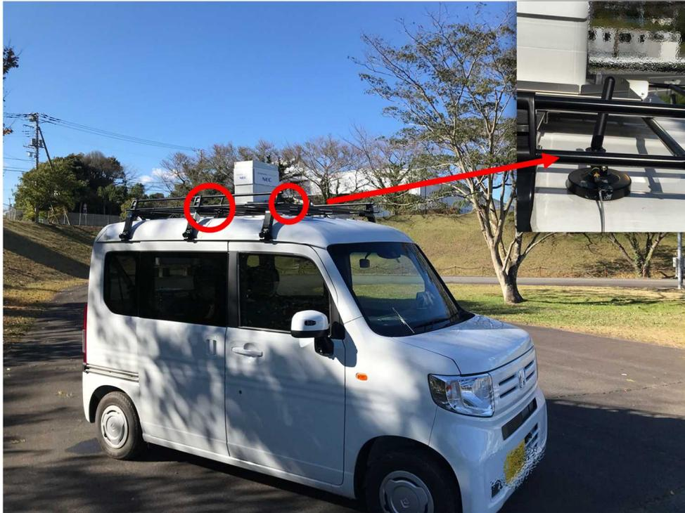
**Fig. 3.4.1-3 Light van equipped with OBU (radio antenna indicated by the red circle)**
