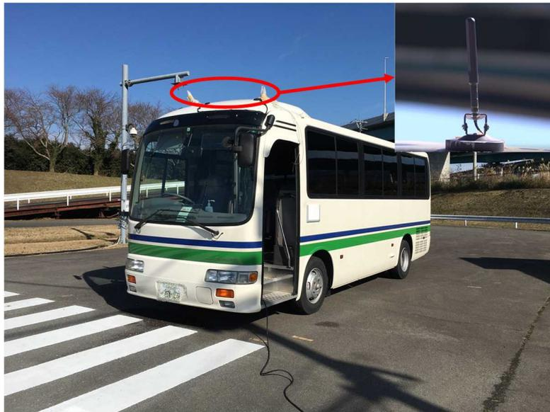
**Fig. 3.4.1-4 Small bus equipped with OBU (radio antenna indicated by the red circle)**
