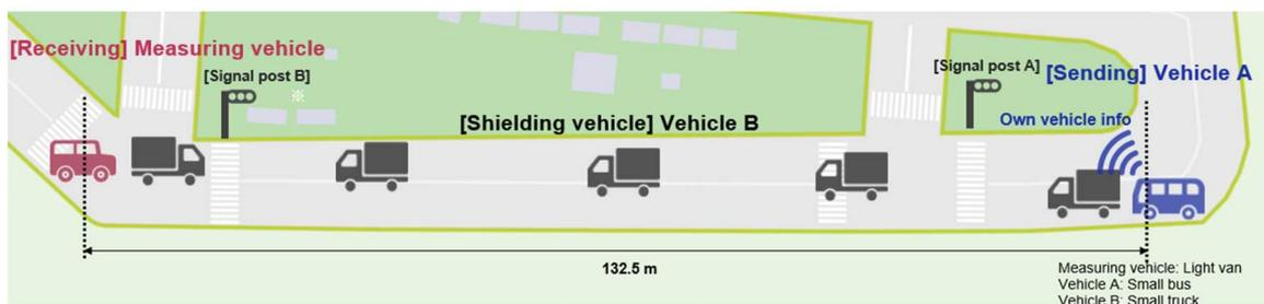
Fig. 3.4.3-1 Overview diagram of Demonstration (1)
