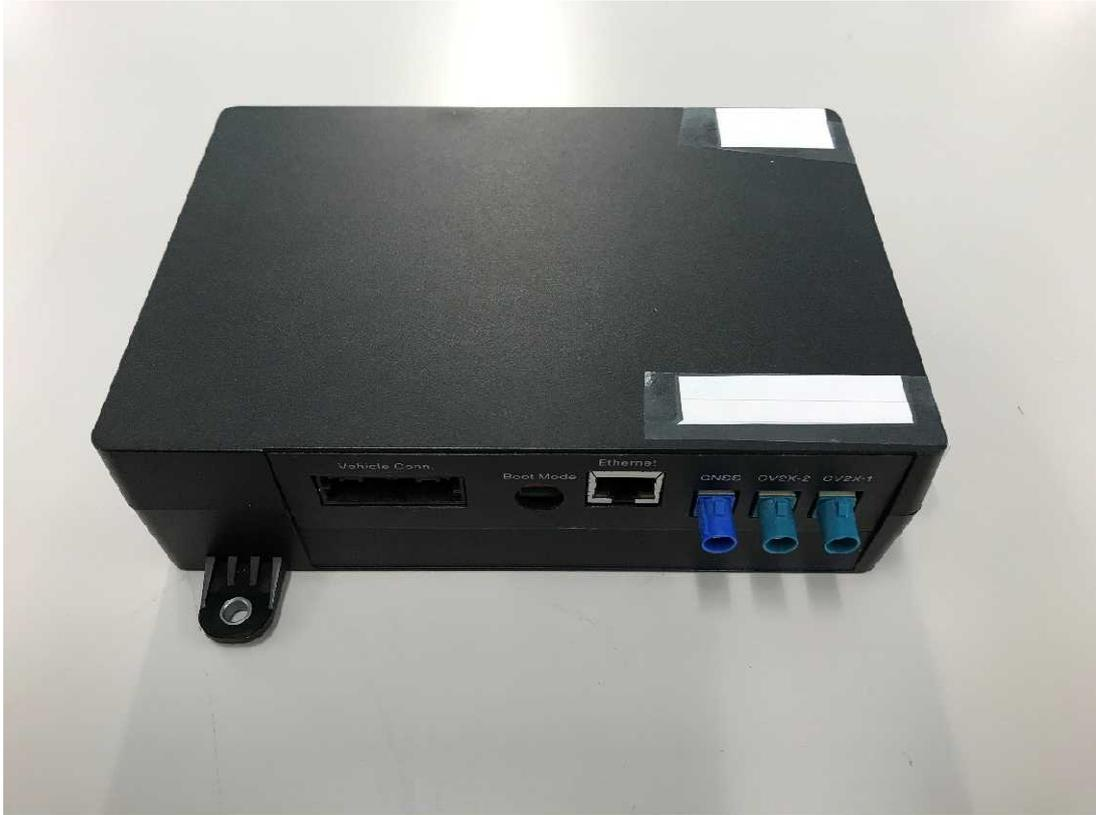
**Fig. 3.4.1-8 C-V2X Unit (made by WNC)**
