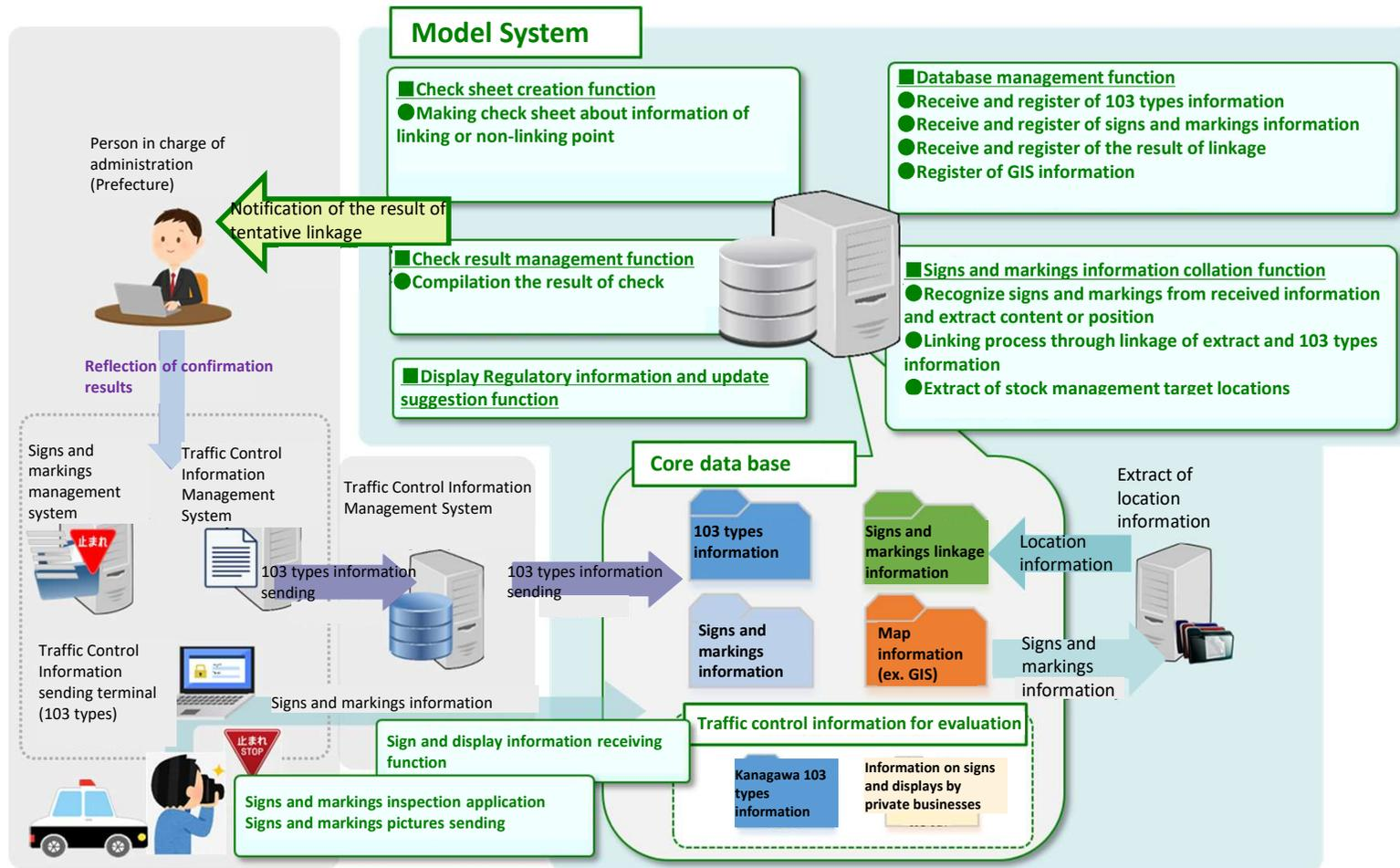
Fig.7. Image of the functional structure of the model system
