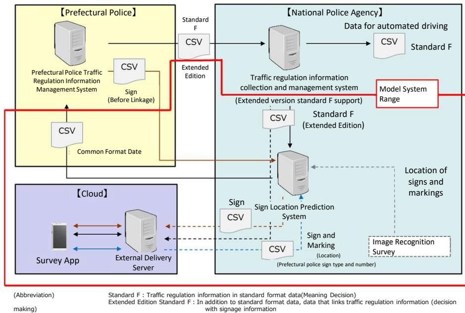
Fig.8. Equipment configuration of the model system
