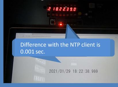
Communication delay from traffic signal controller (Example)
