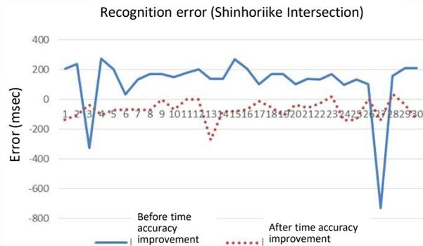
Improved time accuracy was confirmed after installing GPS to the traffic signal controller.
