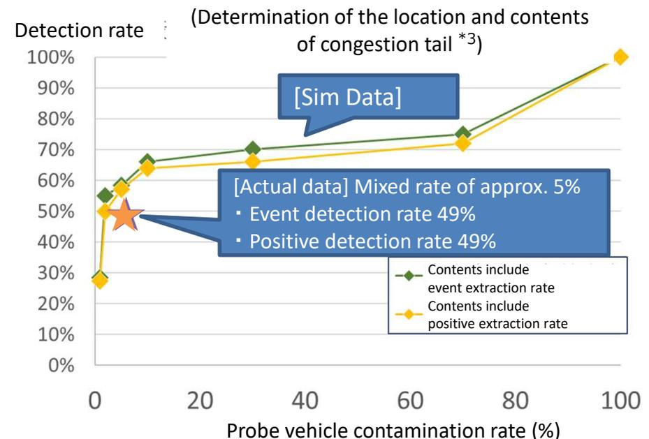
\*1 Probe vehicle contamination rate: 1%, 2%, 5%, 10%, 30%, 70%, Number of judgment samples: 1% and 2% contamination rate ⇒ 2 vehicles, 5% and 10% contamination rate ⇒ 5 vehicles, 30% and 70% contamination rate ⇒ 10 vehicles
