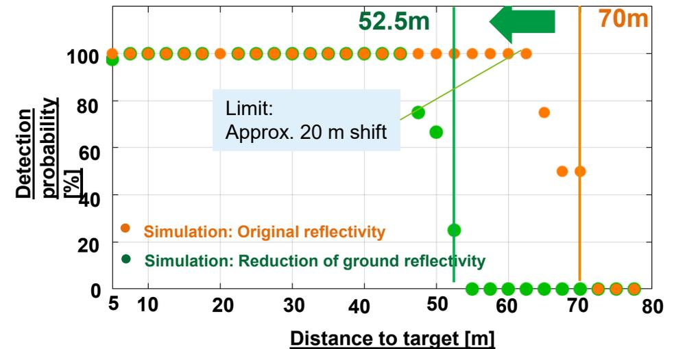
Ground reflectivity differences around the target significantly reduce the target's detection limit for long distance.
