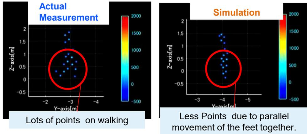
Large difference in the shape of the lower half of the target between actual measurement and simulation
