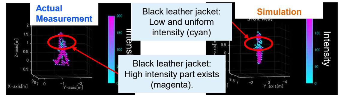
Although black leather jacket have specular components, they are not reproduced in the model ⇒ Candidate of difference factor
