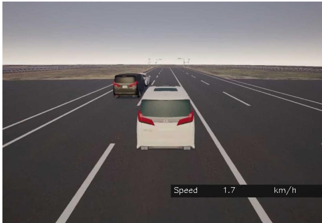
Improved fusion method to correct AEB malfunction. In addition, considering the actual amount of input delay, the AEB is designed so that it will not operate until the timing when a person cannot step in time.
