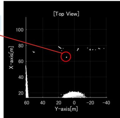
Differences in the detection limit of distant targets due to differences in point cloud around the target
