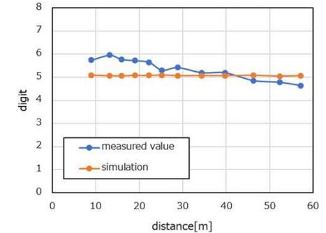
Regarding the noise waveform intensity, there is a challenge in the measurement method (reproduction of background light). Since beam spot size increases with distance, halogen light is not uniformly irradiated on the target within the field of view, which is presumed to be the cause of the inconsistency.
