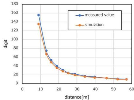
Standard deviation of received signal peak intensity
