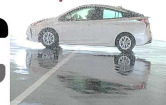
⑤ Occurrence of false points due to specular reflection on wet surfaces
