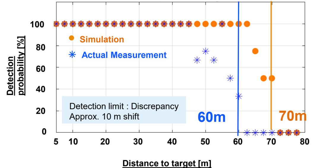
**A large difference of 10 m or more was observed in the detection limit of the distant object of the actual measurement and the simulation.
