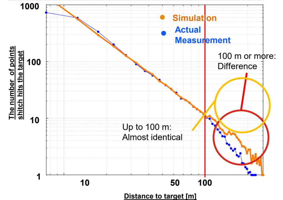
**The reason for the discrepancy in the distant point number is considered to be the difference in the measurement distance limit of LiDAR.**
