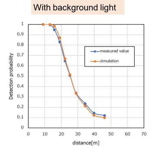
*Confirm consistency of ranging limit (detection probability) by both conditions without background light and with background light.*
