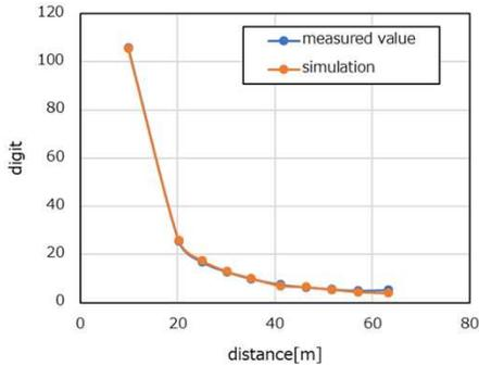
Standard deviation of received signal peak intensity
