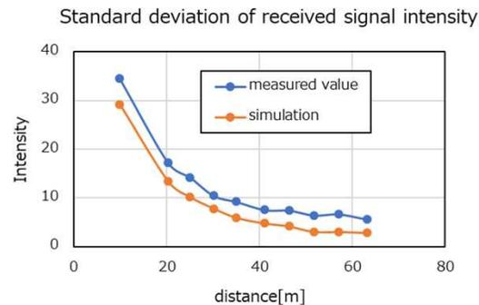
*The differences of accuracy and precision between measured value and simulation are small, and the measured value tends to be higher than simulation.*
