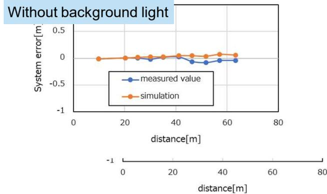
*Adequate consistency was confirmed for accuracy and precision.*
