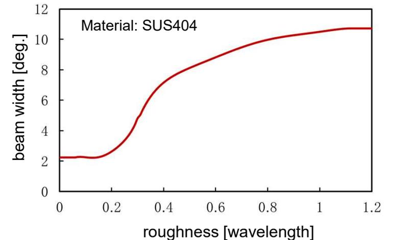
Example) Relationship between surface roughness and reflected beam width
