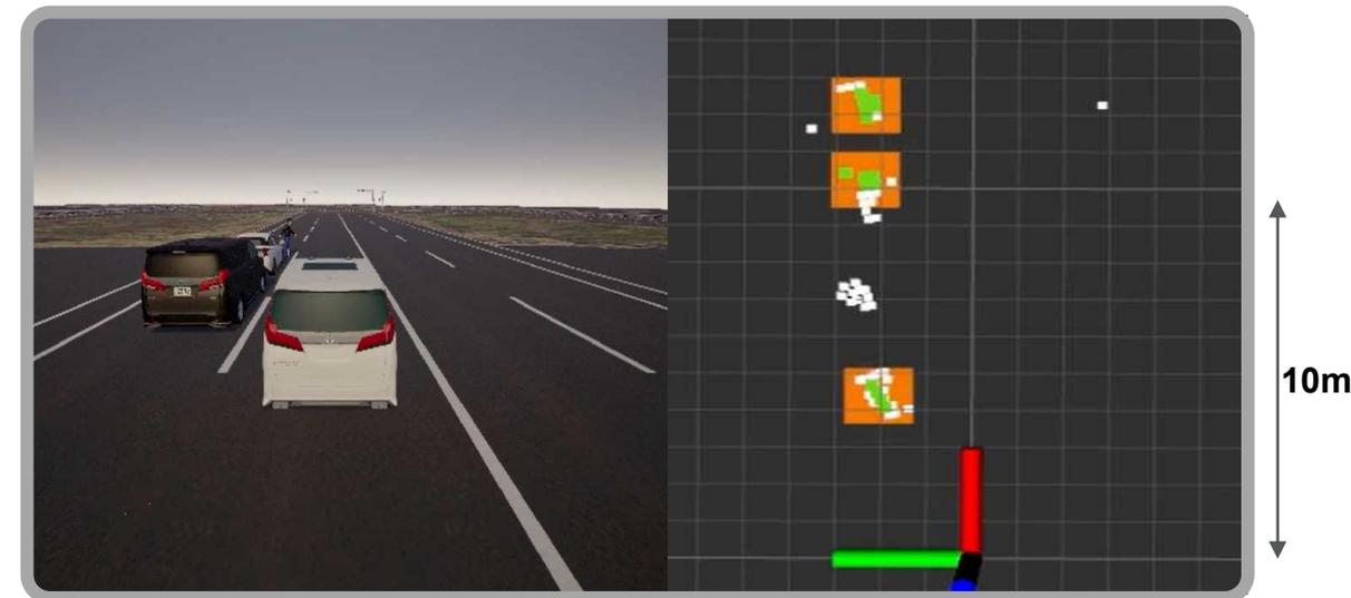
※Simulation conditions : reflector OFF、 number of refraction 1, maximum perception output 200 points
