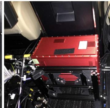
High-precision GNSS vehicle inertial device IMU
