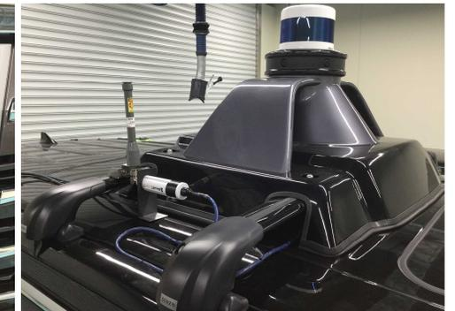
Sensor vehicle-mounted technology for vehicle inspection
