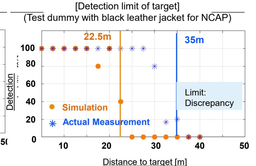
**Confirmed consistency of long-distance detection limit in test dummy for NCAP**
