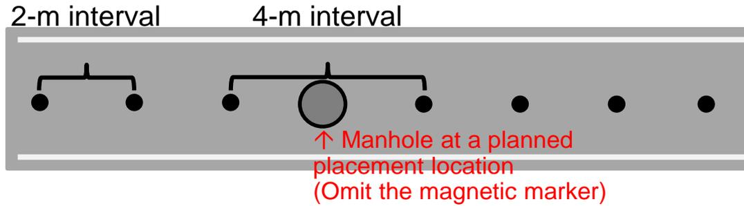
If there is a manhole at the planned placement position of a magnetic marker, the marker is omitted.
