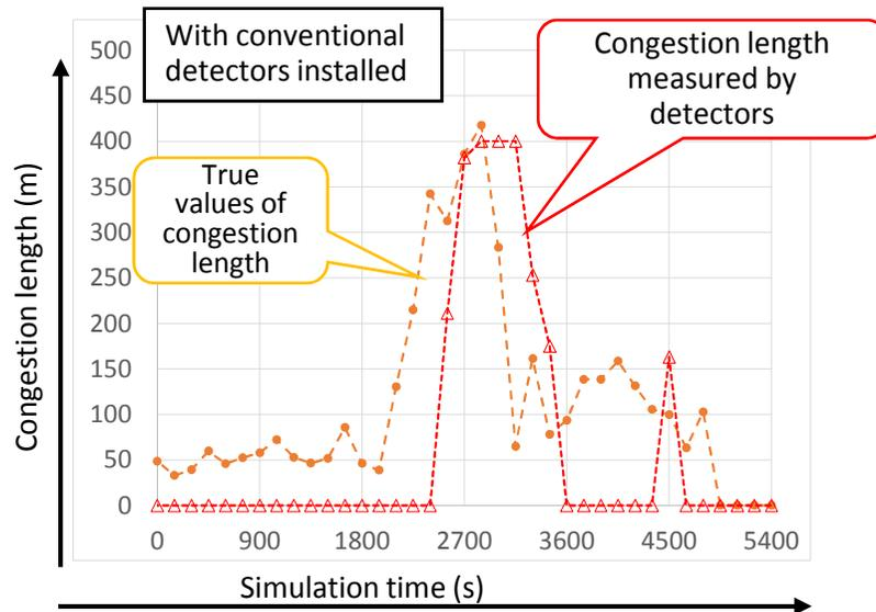
Results of the measurement of a congestion length on a main road (Section 1) with conventional detectors installed
