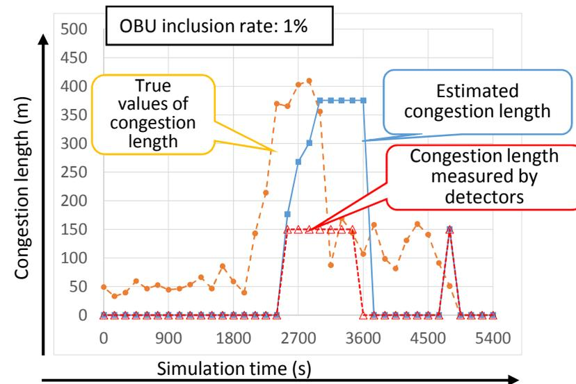
Results of the measurement of a congestion length on a main road (Section 1) under traffic control using fewer detectors
