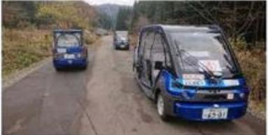
One remote monitor/operator handles operation for 3 unmanned vehicles
