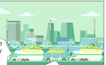
When multiple vehicle operate on the same expressway, they communicate to each other, and system decides whether to form a platoon and when to disengage.
