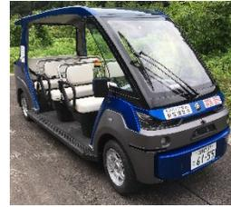
**Smart E cart (Low-speed automated driving vehicle)**
