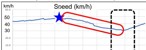
Backlighting caused reduced signal recognition accuracy, so the vehicle automatically slowed down in order to be able to stop. Because the signal was green, the vehicle traversed the intersection and reaccelerated
