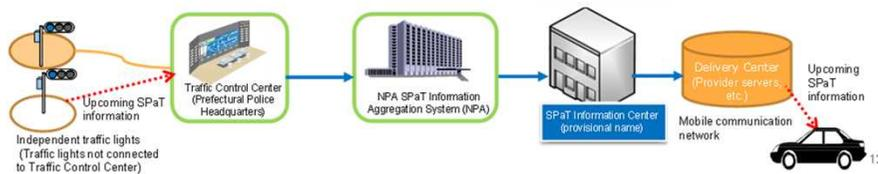
② Traffic signal control using GNSS (location information) and other technologies
