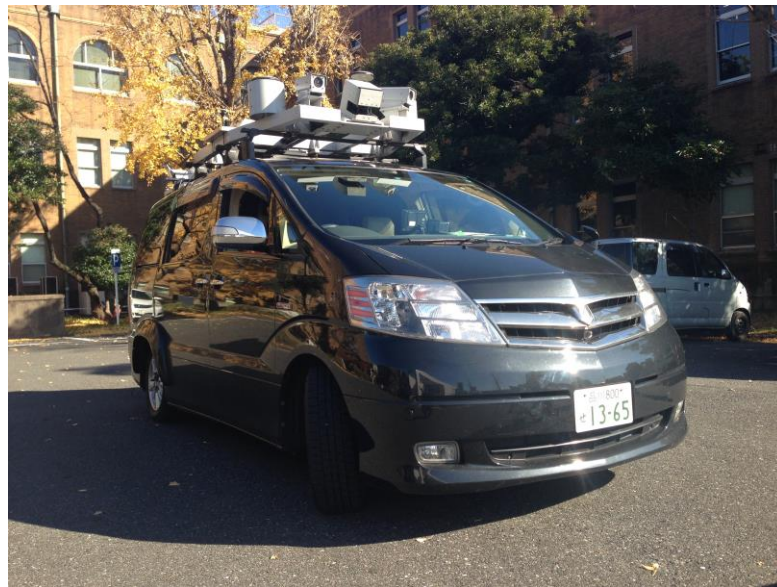
Mobile Mapping System (MMS)
